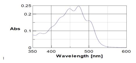
Figure 5: Spectra analysis for particle size (152 micron, 100 BSS) Peak executed – 472 nm Absorbance – 0.24787
