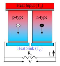
Fig. Arrangement of thermoelectric module for power generation by seeback effect
