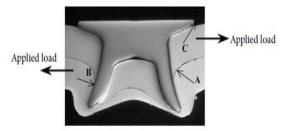
A: interface between the two riveted sheets B: interface between the rivet shank and the locked sheet C: interface between the edge of the rivet head and the pierced sheet
