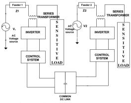
Fig.1. Interline dynamic voltage restorer
