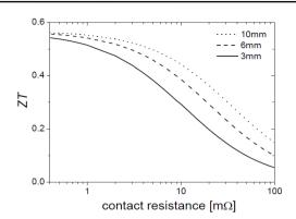
Figure no. 7:- Impact of the contact resistance on the ZT-value of the module for modules with different leg sizes, calculated at room temperature [3].
