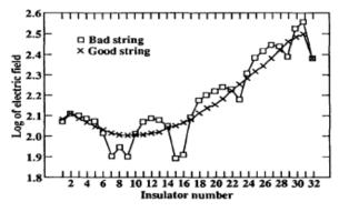
Fig: 6 Log of electric field Vs Insulator no. [10]
