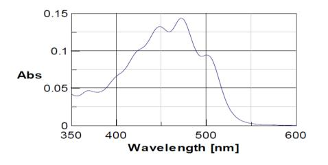
Figure 2: Spectra analysis for particle size (297 micron, 52BSS) Peak executed – 472 nm, Absorbance – 0.14411
