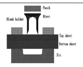
Fig.7.- FE model of SPR process
