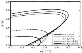
Figure No.5: Effect of heat transfer law on power output versus efficiency. [2]
