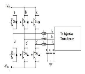
Fig.2. Three-leg voltage source inverter
