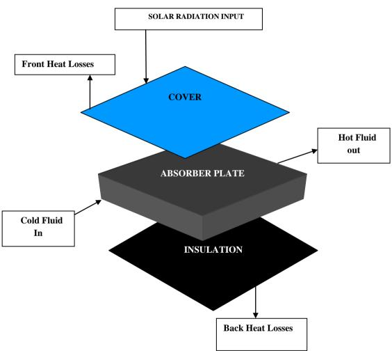
Figure 1: The Flat Plate Solar Collector
