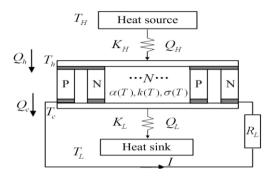
Figure 1:- The finite time thermodynamic model of an irreversible multi-element thermoelectric generator with external heat transfer. [2]
