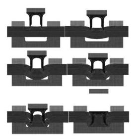
Fig.8 Simulation of SPR process
