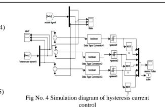
The switching signals thus generated are fed to the power circuit which comprises of a three phase three leg VSI with a DC link capacitor across it. Based on these switching signals the inverter generates compensating current in phase opposition to the line current. The compensating current is injected back into the power line at the PCC and thus suppressing the current harmonics present in the line. The overall simulation block diagram is shown in Fig 5.
