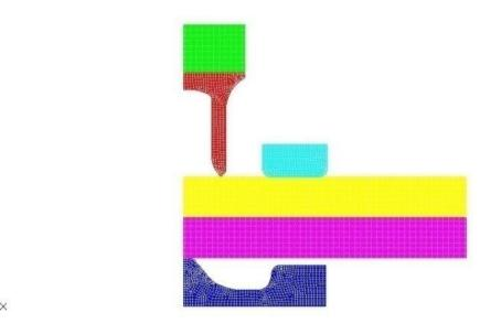
Fig. 9- FE Model for SPR Process
