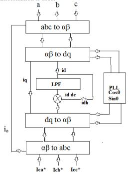
Fig No.2 Block diagram of SRF based algorithm
