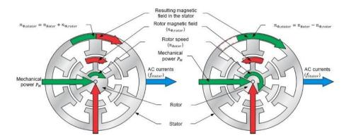
Fig.2 DFIG wind turbine rotating magnetic field representation
