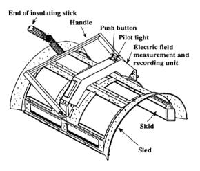
Fig: 5 Insulator tester [10].
