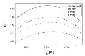
Figure no. 8:- The modules ZT-values versus the cold-side temperatures Tk for different leg sizes. The simulations predict, that modules with longer legs show a better performance [3].
