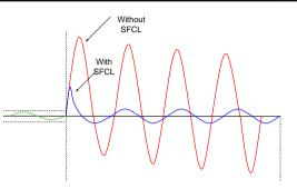
Fig.1: Fault current waveform with SFCL and without SFCL
