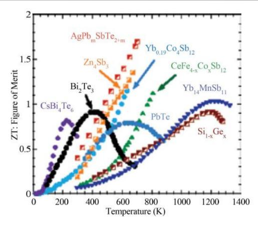
Figure 3. Figure of merit (*ZT*) as a function of temperature for several high-efficiency bulk thermoelectric materials [14].
