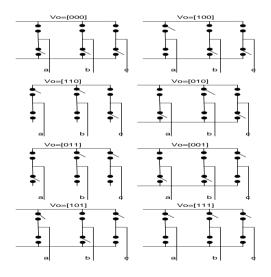
Fig.3. eight switching states of inverter
