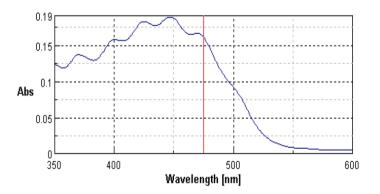
Figure 6: Spectra analysis for particle size (125 micron, 120 BSS) Peak executed – 472 nm Absorbance – 0.18927
