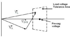
Fig.6 Voltage Tolerance Method
