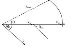
Fig.5 In Phase Compensation Method
