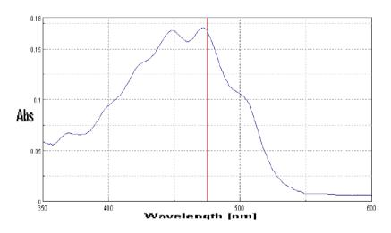
Figure 3: Spectra analysis for particle size (251 micron, 60 BSS) Peak executed – 472 nm, Absorbance – 0.17058
