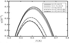
Figure No.3: Effect of heat transfer law on efficiency versus working electrical current. [2]
