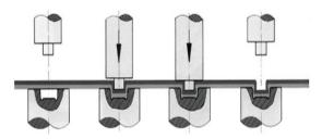
Fig.4: Principle of mechanical clinching
