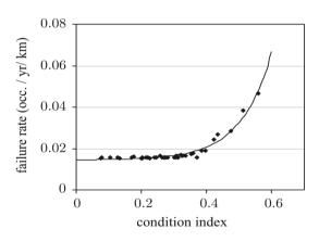
Fig.16: Relation of condition index and failure rate of overhead lines [1].
