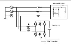
Fig No.1 3- phase shunt active power filter with SRF controller
