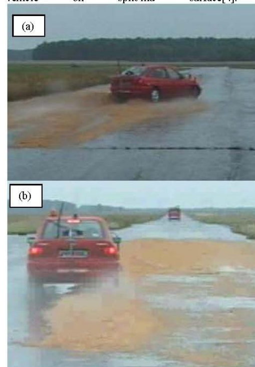
Fig. No.1: Vehicle stability on split- \mu surface during braking on wet asphalt covered with grain: (a) without ABS, (b) with ABS [4]
