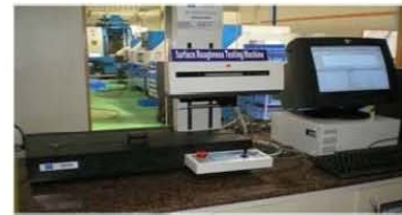
Fig. No.2 Equipment for Surface Roughness Measurement
